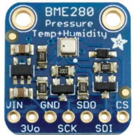
Bosch's BME280 measures air pressure, temperature and humidity in one.
