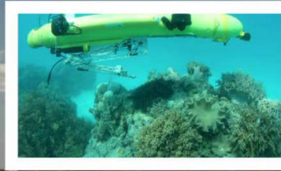
The COTSbot identifies the Crown of Thorns Starfish with machine learning. (Source: Queensland University of Technology)
